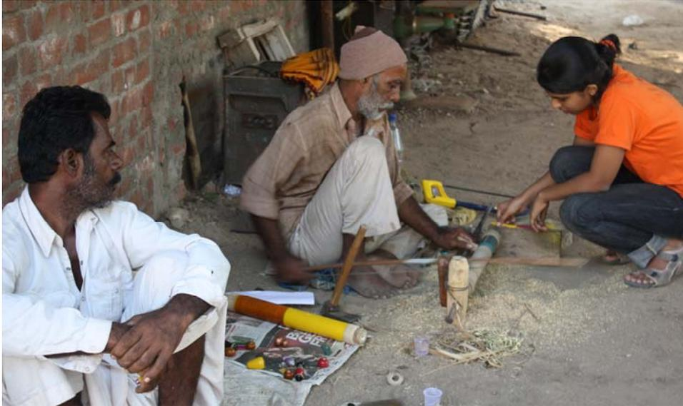
Figure.1 Poorva K. from NID working with craftsmen to turn solid bamboo on a traditional lathe
